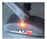
(11) Note that it may take up to 20 seconds for the GPS to establish a signal lock. When the signal is locked, an LED indicator begins flashing on a 1 second interval at the location shown below
